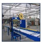
The CI 89 Y is a reliable automatic strapping machine, with a site seal. Because of the easy varity in strap tension (up to 800 N), the CI 89 Y is suitable for many different products. The automatic strappingmachine CI 89 Y is available for many branches. This machine is perfectly suitable to build in automatic processing lines.
